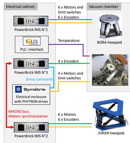
Figure 4: Hardware architecture.
