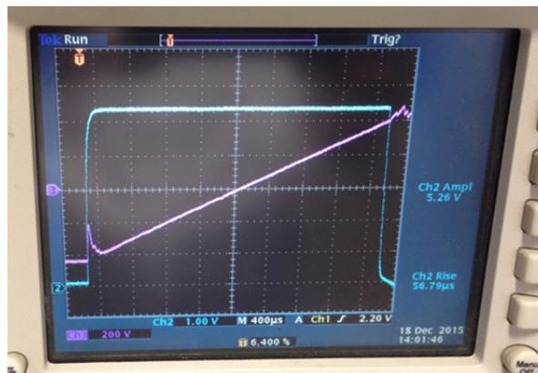
Figure 4: Regulator voltage during a klystron pulse. Ch 2 (blue) shows pulse voltage, 20 kV/div, 400  $\mu$ s/div. Ch 3 (pink) shows regulator voltage, 200V/div, 400  $\mu$ s/div. The pulse settles rapidly and remains extremely flat (< 0.1%) over the long pulse flat top (3.5 ms).
