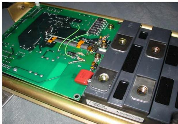
Figure 10. IGBT module and gate driver.
