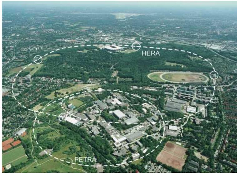
**Figure 3.1:** An aerial view of DESY. The dashed lines show the underground locations of the PETRA and HERA ring accelerators as well as the location of the four large HERA detector halls (north, south east, west). The DESY site is encircled by the PETRA ring. The HERA facility runs under Hamburgs Volkspark as well as beneath residential and industrial areas of the city.
