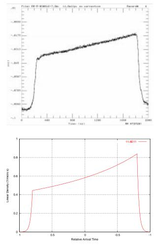
Figure 12: The observed longitudinal profile of a  $11.8 \times 10^{11}$  beam in the top plot is very linear, whereas the theoretical predicted profile assuming Gaussian energy distribution in the lower plot is not.
