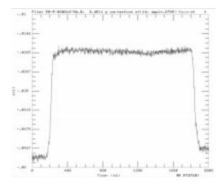
Figure 9: The head-tail asymmetry of the beam profile in Figure 7 is compensated by adding  $\sim 8.82$  V to the region between the barriers.
