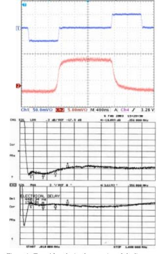
Figure 5: Top: A beam of intensity  $\sim 1 \times 10^{11}$  exhibits head-tail asymmetry between two barrier waves. Middle and bottom: Amplitude and phase in the Recycler highlevel rf exhibit nonlinearity from 90 kHz to 1 MHz. The amplitude plot is 0.2 dB per division and the phase plot is 2° per division. Markers 1 and 2 are at fundamental (~ 90 kHz) and first (~ 180 kHz) revolution harmonics. A response with flatness of less than 0.26 dB in amplitude and less than 1.8° in phase is required.
