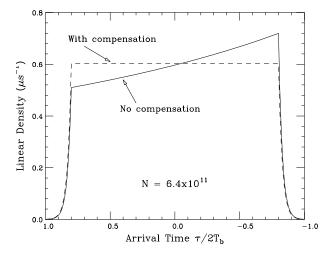
Figure 8: Solution of the Haissinski equation [Eq. (9) below] with a resistive impedance of  $R_s = 200 \ \Omega$  and beam intensity  $6.4 \times 10^{11}$  reproduces the observed beam profile with head-tail asymmetry shown in Figure 7. A compensating voltage, 12.4 V, restores the head-tail symmetry. Here  $T_b$  is total bunch length.
