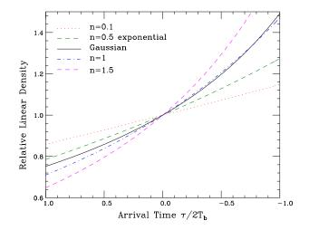
Figure 13: Longitudinal beam profile in the generalized elliptical distribution. Starting on the left from the top and going downward, the longitudinal beam profiles correspond to n = 0.1, n = 0.5 (exponential), Gaussian, n = 1.0, and n = 1.5. The predicted beam profiles are quite linear when  $n \leq 0.5$ . Here,  $T_b$  is total length of beam.
