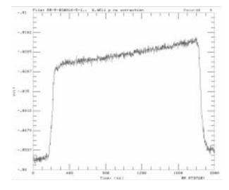
Figure 7: A beam of intensity  $N = 6.4 \times 10^{11}$  inside a barrier bucket of width  $\sim 1.59 \ \mu s$  exhibits head-tail asymmetry, after response linearization is implemented. The beam lags backwards in agreement with energy loss due to resistive impedance.
