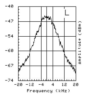
Figure 14: Schottky signals of the 19485th revolution harmonic (1.75 GHz) of a beam of intensity  $11.67 \times 10^{11}$ in a barrier bucket. The Schottky amplitudes are in dBm which is defined as  $10 \log_{10} N_i / N_0$ , where  $N_i$  is the amplitude at the *i*th point and  $N_0$  is a scale factor.
