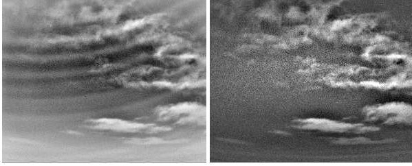
Figure 1: Left: Raw image from a field-of-view sequence taken from Coihueco on 2009/07/19 at 08:25 UTC. Right: The same image after having a clear sky template image removed from it. A signal threshold is then applied to create a binary cloud mask which is then mapped to the FD telescope pixels.
