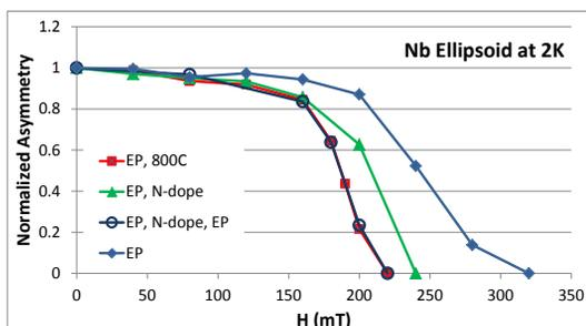
Figure 12: Ellipsoid samples treated at EP+800C and with N-doping compared to no heat treatment (Ep only).
