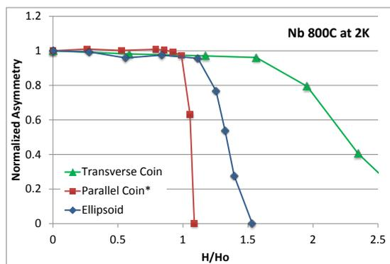
Figure 7: Similar to Fig. 6 but with samples treated at 800°C (parallel coin is N-doped at 800C and then given an EP of 5 $\mu$ m) showing sensitivities of different geometries to pinning.
