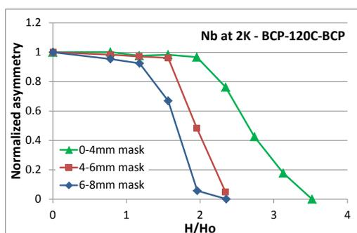
Figure 8: Field entry as a function of position on the sample for transverse coin geometry for a sample with a treatment of BCP-120C bake-BCP.
