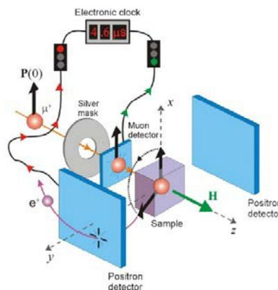
Figure 1: TF- $\mu$ SR setup with the initial muon spin polarization perpendicular to the magnetic field. The silver mask in front of the sample restricts the muon implantation to the central region of the sample.
