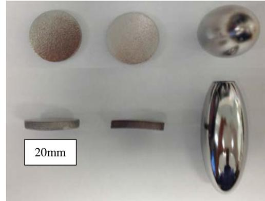
Figure 3: Example of the samples used in the experiment: plan view and side profile for flat coin, formed coin and ellipsoid.
