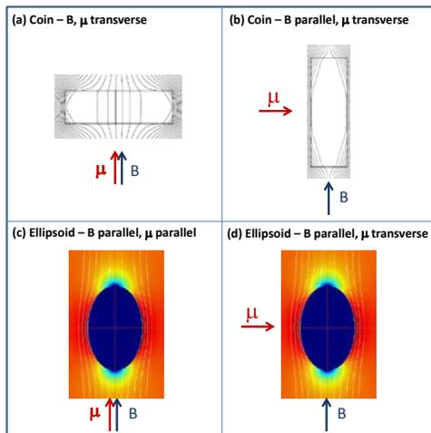
Figure 2: Four generic arrangements of sample (coin and ellipsoid), muon and field direction for the sample characterization studies at TRIUMF.
