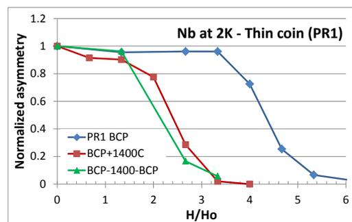
Figure 9: Results from transverse coin sample (PR1 – 0.8mmx16mm) after BCP treatment followed by annealing (1400C) followed by another BCP.
