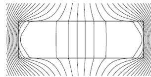
Figure 4: Flux applied to a thin circular disk transverse to an applied field where  $H_{applied} > H_{applied}^{entry}$ .
