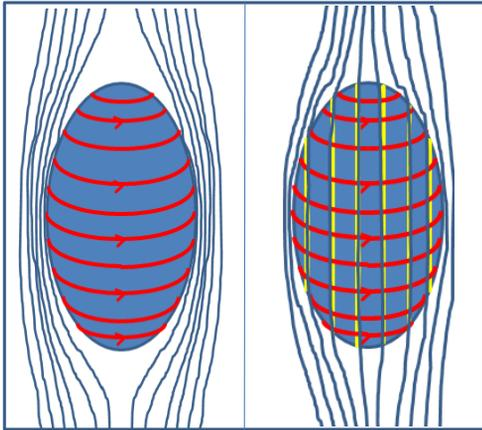
Figure 5: Schematic showing the magnetic flux just before and after flux nucleation at the ellipsoid equator.
