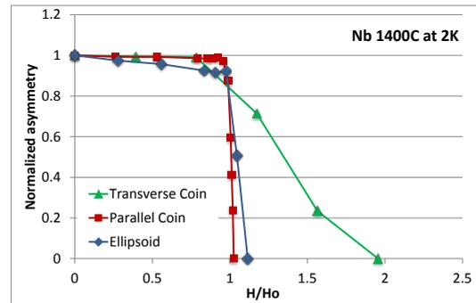
Figure 6: Normalized asymmetry plots showing fraction of sampled volume devoid of magnetic field as a function of applied field normalized to the expected  $H_{applied}^{entry}$  based on the demagnetization factor of the geometry. Shown are plots for samples annealed at 1400C to reduce pinning - a coin in transverse and parallel geometry and an ellipsoid with geometry as in Fig. 2c.
