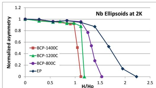
Figure 11: Ellipsoid samples heat treated at 1400C, 1200C, and 800C respectively for four hours each assuming  $H_{nucleate|0K}=180mT$ .
