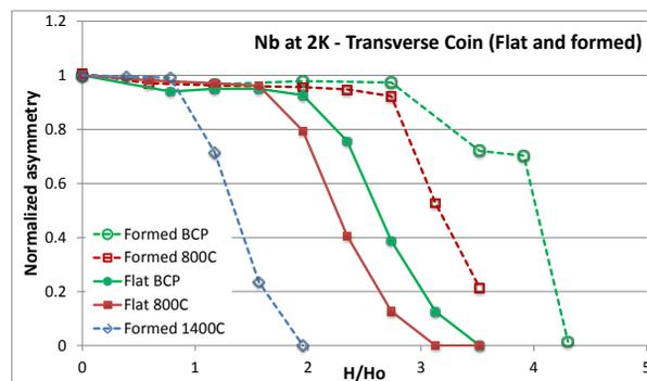
Figure 10: Results from transverse coins of formed and flat geometries. Formed samples are denoted with dashed lines. Red lines are samples treated at 800C for 4 hours; green lines are for samples after BCP; blue line is a sample annealed at 1400C.
