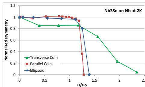
Figure 13: Coin and ellipsoid sample results at 2K for a 2μm coating of Nb<sub>3</sub>Sn onto Nb.
