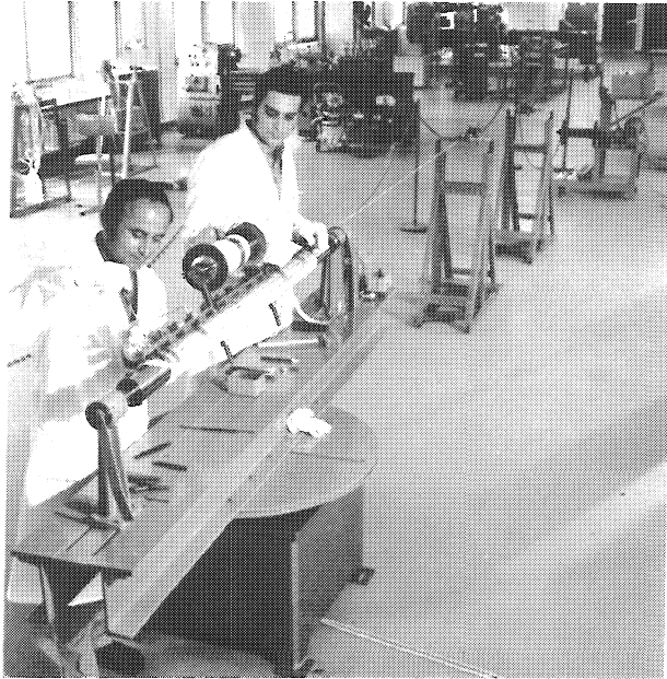
Fig. 13 Trial coil winding of D2a (IEKP). Over-all view and detail
