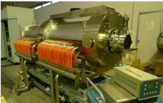
Figure 14: The ferrite-loaded cavity under test.
