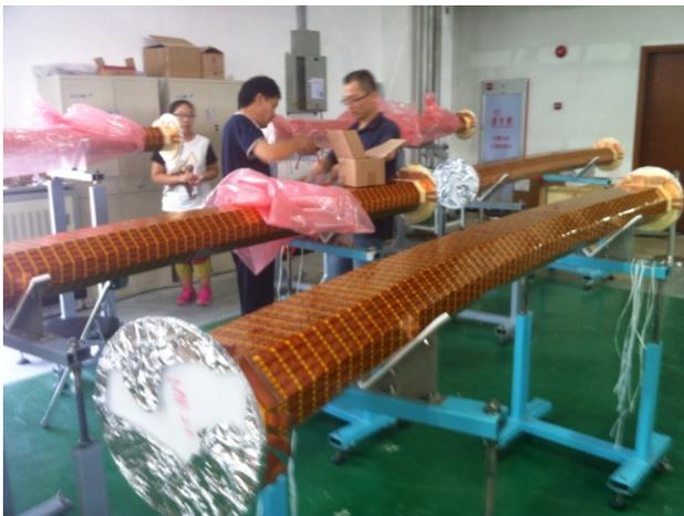
Figure 15: The ceramic chamber for dipole.
