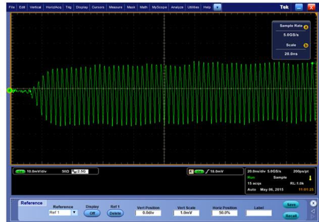
Figure 5: The waveform of beam, in which the rise time of chopper can be investigated.
