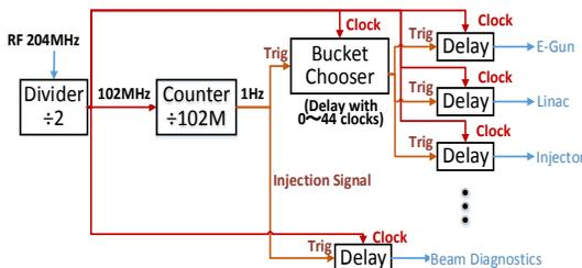
Figure 2: The functional diagram of the timing system.
