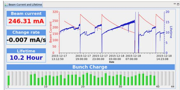
Figure 4: Injecting bucket by turns in decay mode.
