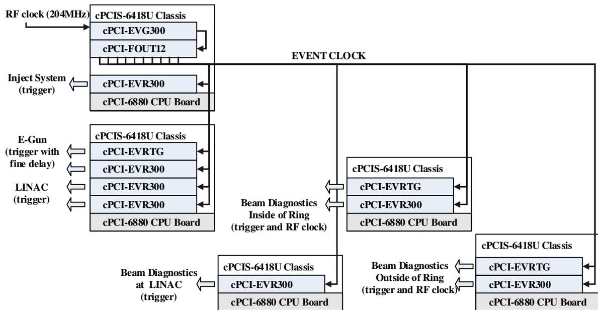
Figure 1: Overview of the HLS-II timing system.
