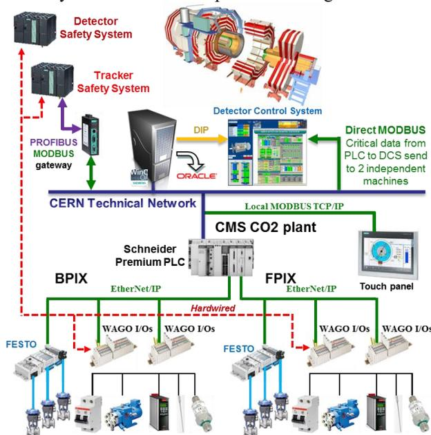
Figure 1: CMS CO<sub>2</sub> cooling control system architecture.
