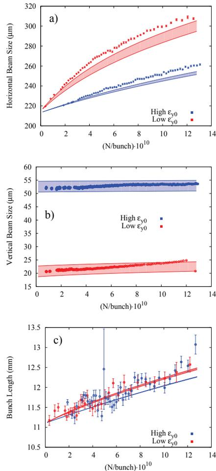
Figure 2: Measured and computed (a) horizontal size, (b) vertical size, and (c) bunch length for a 2.3 GeV bunch of positrons.
