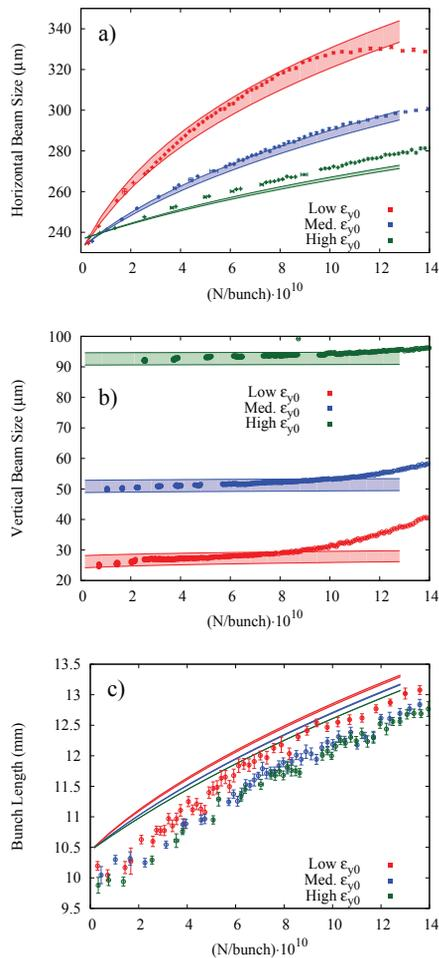
Figure 1: Measured and computed (a) horizontal size, (b) vertical size, and (c) bunch length for a 2.1 GeV bunch of electrons. Points are data, shaded bands are calculated beam sizes reflecting the uncertainty in the zero current vertical emittance.  $N$  refers to number of particles.
