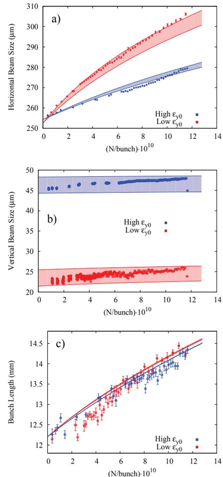
Figure 3: (a) horizontal, (b) vertical and (c) bunch length measurements and simulation results from 2.5 GeV e<sup>+</sup> bunch.
