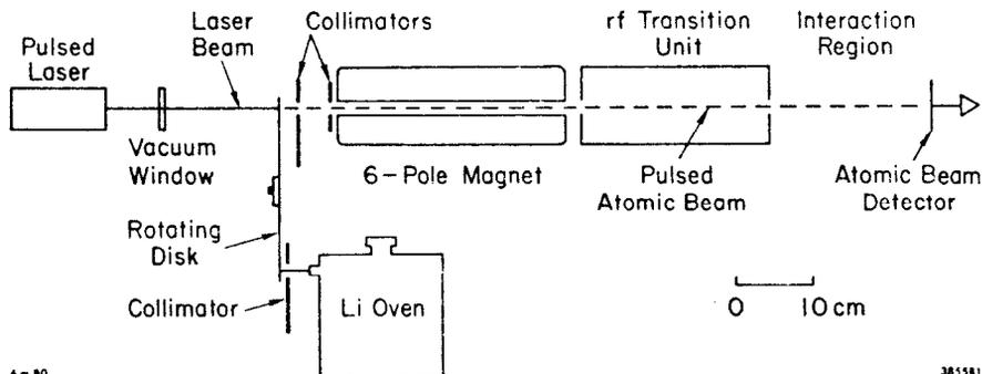
Fig. 1. Schematic diagram of pulsed beam polarized target. The dimensions are to scale except the i.d. of the beam defining orifices are as follows: oven orifice and oven beam collimator, 1.7 mm and 2 mm; laser beam (o.d.), pulsed beam collimators (2), and magnet gap, 2 mm, 2.2 mm, 3.8 mm, and 6.3 mm.
