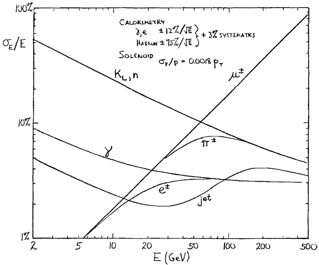
Fig. 6. Energy resolution calculated for various types of particles to be detected in a large solenoid detector system (Ref. 4).
