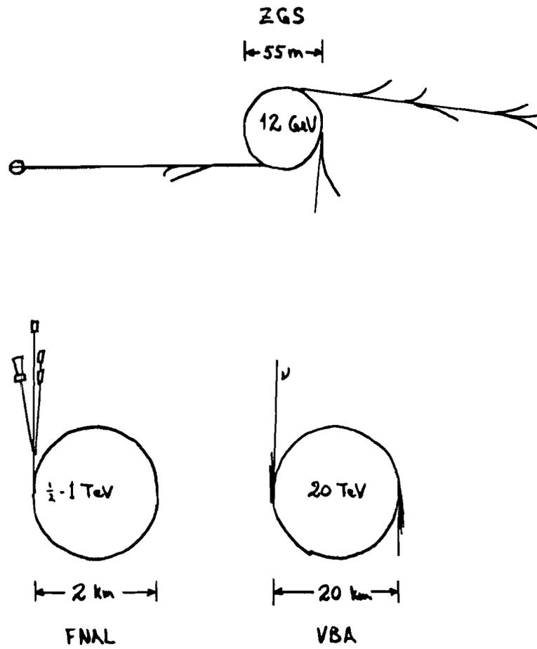
Fig. 5. Site plans for three laboratories, showing that the external beam lines become a relatively smaller part of the laboratory as the energy increases.
