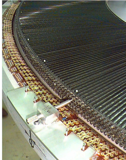
Figure 1.9: Photograph of a four-plane TRT endcap wheel during assembly.
