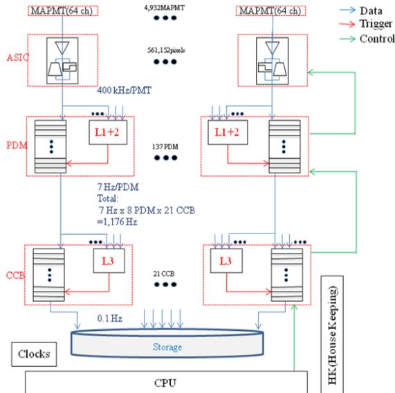
Figure 1. JEM-EUSO trigger, readout and control architecture.
