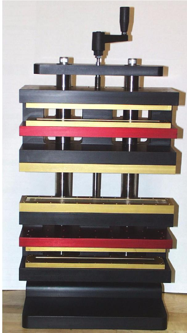
Figure 6: Prototype counterforce system. The black jaws hold the main magnets (gold keepers in center) and the moving counterforce magnets (gold keepers at bottom and top). The red fixtures hold the stationary counterforce magnets. The lead screw is 12.7 mm diameter with a pitch of 0.787/mm. The crank handle is 65 mm from axis to handle axis.
