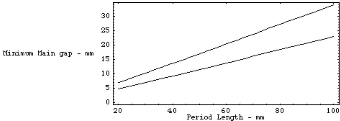
Figure 3: The minimum main gap allowed by the demagnetization of ferrite magnet material, with  $B_r = 0.37$  T and  $H_c = 325$  kA/m. The upper curve is for the case of counterforce and main arrays of equal width and the lower curve is for counterforce magnets twice as wide as the main magnets. Both curves assume magnets with square cross section.
