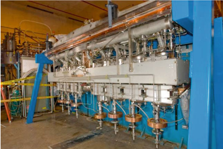
Fig. 1.13 Components suspended from the upper plate of the ALTAS upgrade cryomodule [27]
