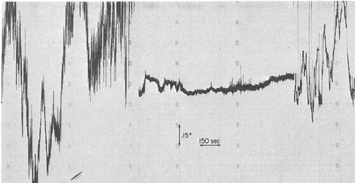
Fig. 5.--Phase stability as function of time. (a) Left: phase measured with unregulated cyclotron. (b) middle: regulated cyclotron. (c) right: The phasemeter itself.
