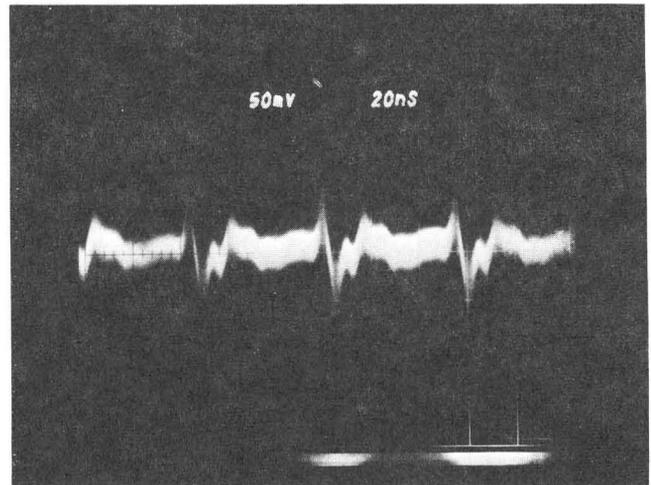
Fig. 2.--Typical signal from the phase-probe for a beam current of 0.6 A.
