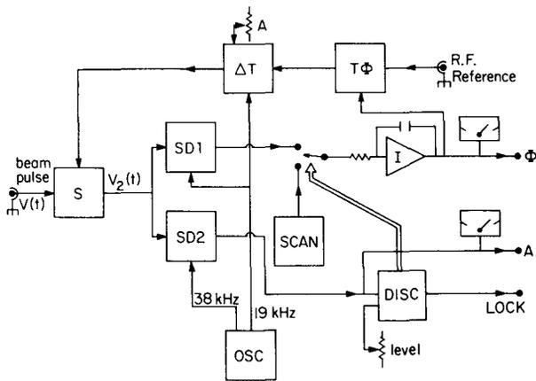
Fig. 3.--Block diagram of the phase-meter.
