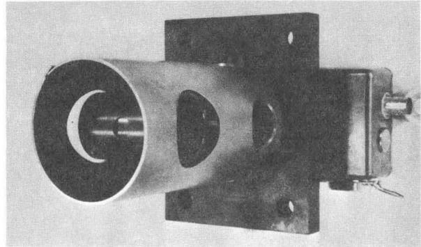
Fig. 1.--Capacitive phase-probe with pre-amplifier.
