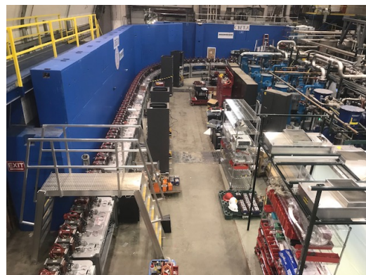
Figure 2: Photo of the straight section of the permanent magnet FFA return loop.
