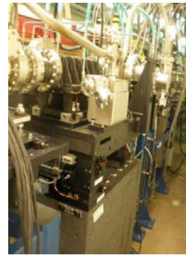
Figure 1: Installed GRID-XBPM at 27-ID FE (Looking upstream) [2].
