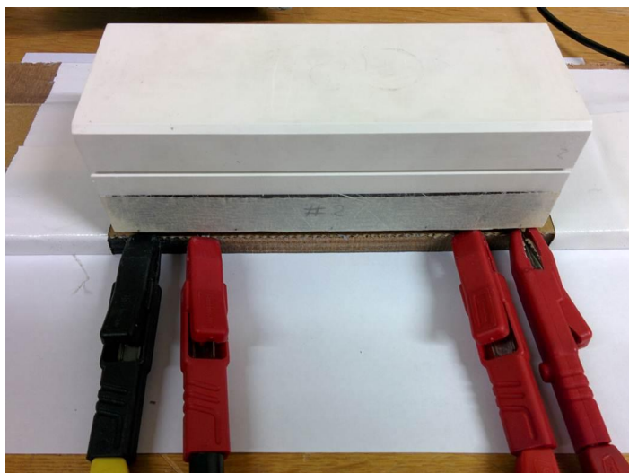
Figure 3.5: Four-pin setup with the block flipped on it.
