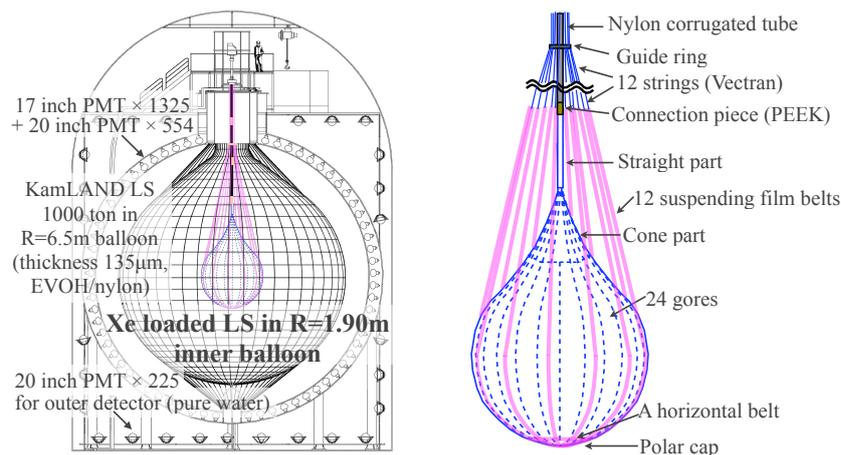
**Figure 1.** Schematic diagram of KamLAND-Zen detector (left) and inner balloon (right).
