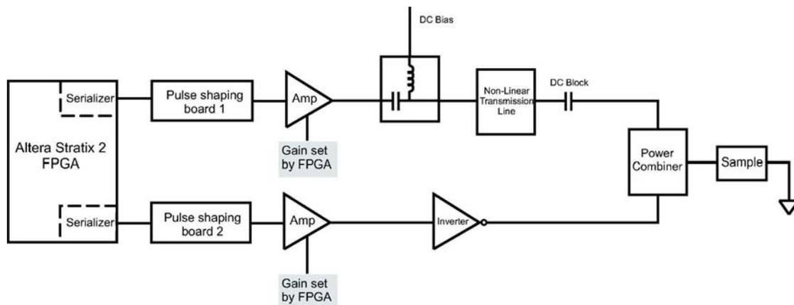
FIG. 4. (Color online) Schematic showing configuration for generating bipolar pulse patterns. Two pulse shaping boards are used. Along one path (bottom), the pulse is inverted. Along the other path (top) the pulse is compressed through a nonlinear transmission line. Pulses are combined in a resistive rf power splitter.
