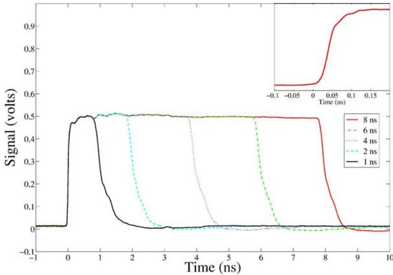
FIG. 3. (Color online) Resulting wave form output from the pulse generator for pulses of width 1, 2, 4, 6, and 8 ns. Inset shows the rising edge of the pulse.
