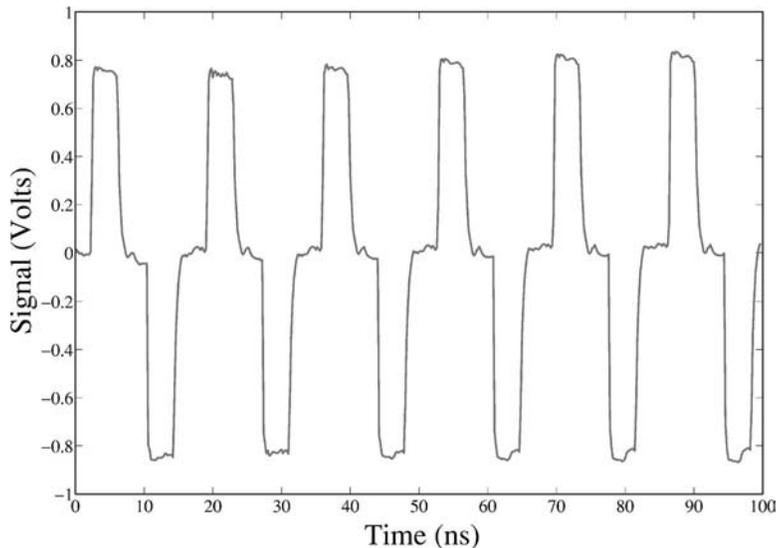
FIG. 5. Pattern of positive and negative pulses at 62.5 MHz.
