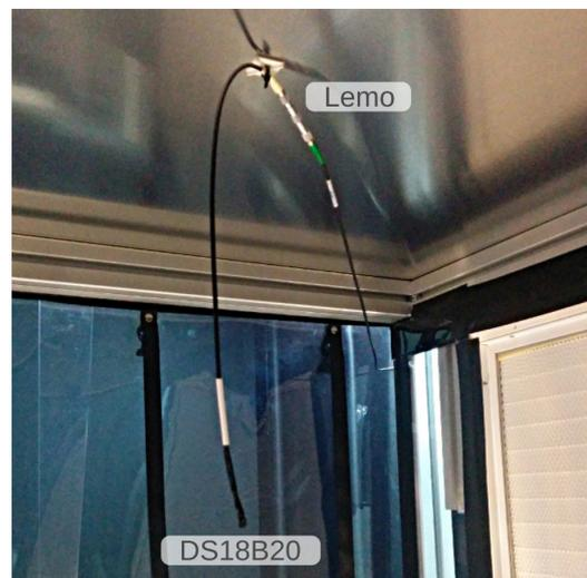
(b) Sensor equipped with a Lemo® connector and deployed above a laser table.
