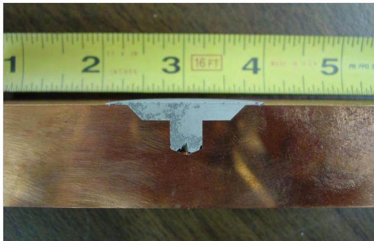
Figure 6.8. Cross section of magnesium friction-welded flange.
