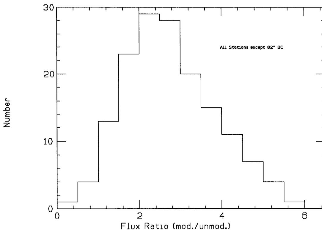
Figure 5. Frequency of moderated/unmoderated neutron ratios.
