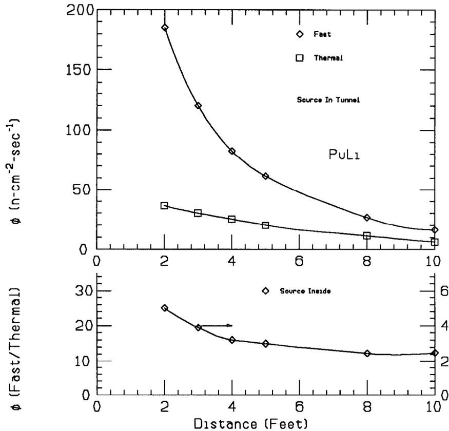
Fig. 7c-d. Mapping of Tunnel Neutrons.
