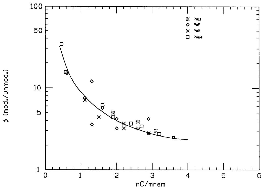
Figure 8. Sensitivity of TLD's versus mod./unmod. fluence ratios.
