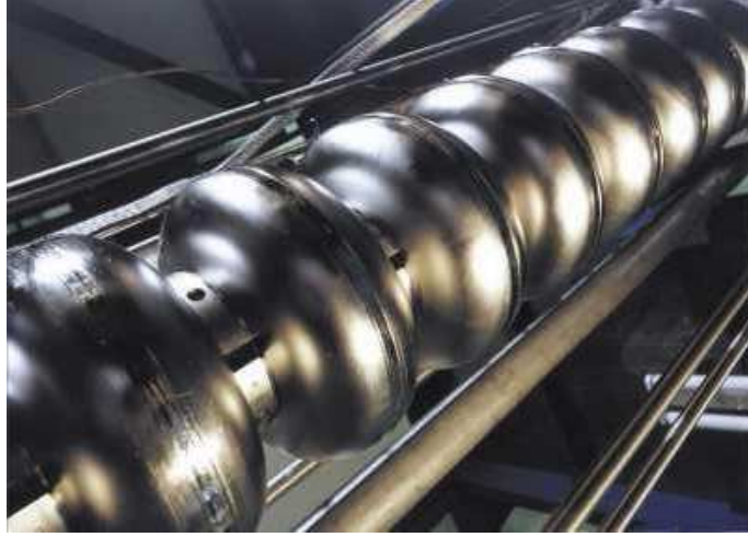
Figure 3.1: Nine cell superconducting niobium cavities operated at a frequency of 1.3 GHz RF as envisaged for the accelerating structures of the International Linear Collider, ILC. The length of the cavity is approximately 1 m.
