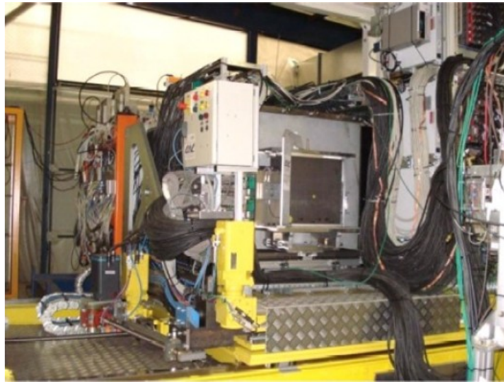
Figure 3.14: CALICE beam test setup in the MTBF area at Fermilab. The SiW Ecal physics prototype is visible in the front, followed by an analogue Hcal and a Tail Catcher and Muon Tracker.
