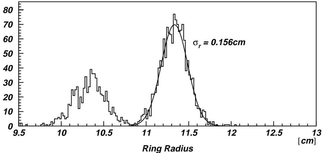
Fig. 4. Ring radius distribution for interaction data for tracks with 95 – 105 GeV/c momentum. Very well separated peaks corresponding to pions (right) and kaons (left) can be seen.
