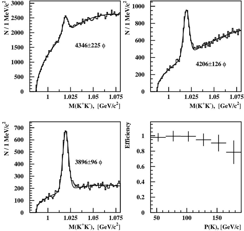
Fig. 3. Invariant mass of  $K^+K^-$ . Top left: No identification of the kaons. Top right: One kaon is identified. Bottom left: Both kaons identified. Bottom right: Efficiency for the RICH to identify a kaon as a function of its momentum. For identification, the likelihood of the track to be a kaon is required to be at least as big as the likelihood of it to be a pion.
