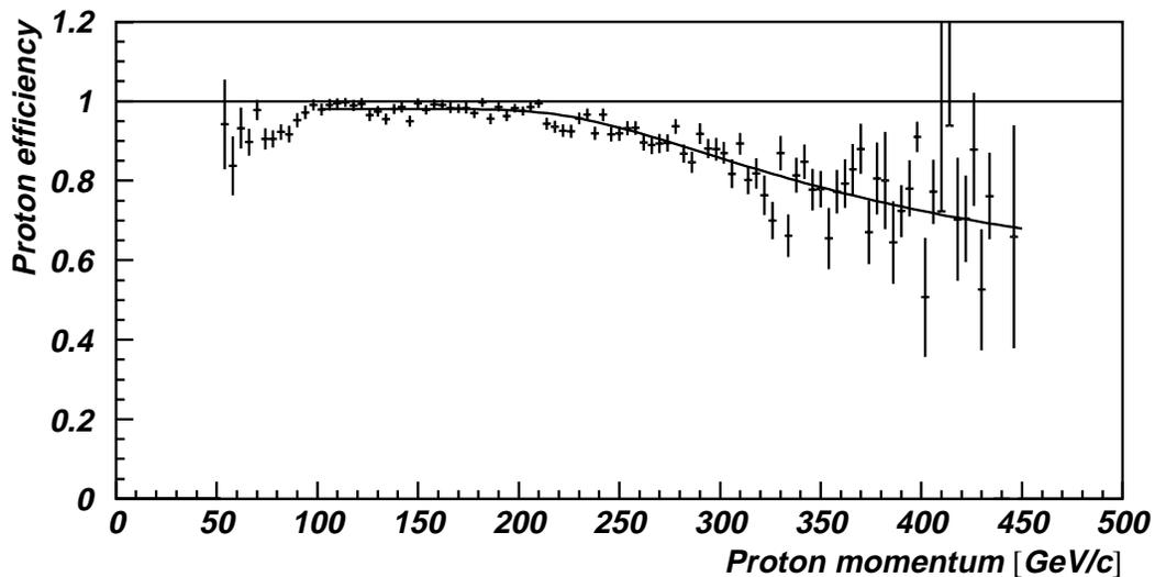
Fig. 5. Proton identification efficiency as a function of the proton momentum.
