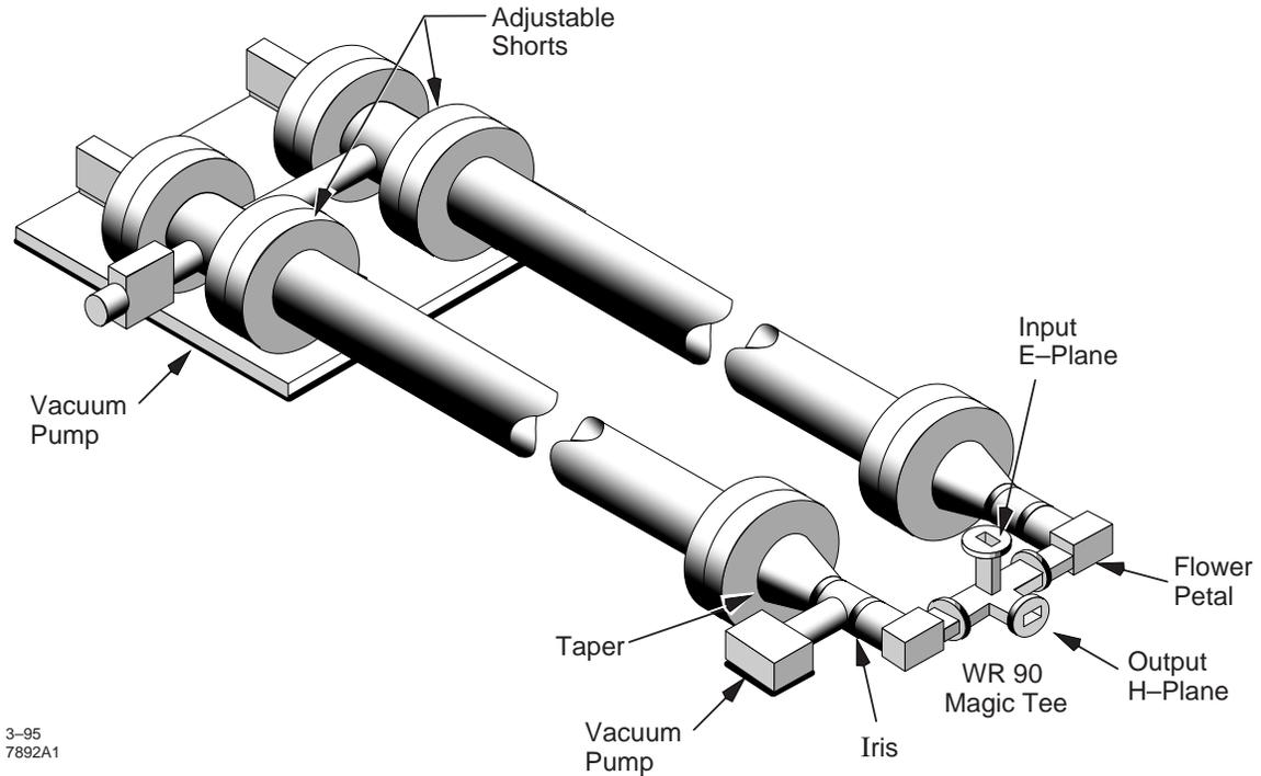
Figure 1. SLED-II layout. Tested with 12.065 cm diameter waveguide, 22.5 m in length (150 nS round-trip rf transit time.)
