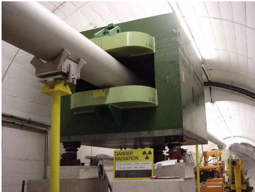
Figure 3.5: The dipole magnet sweeps the charged particles off the beam.
