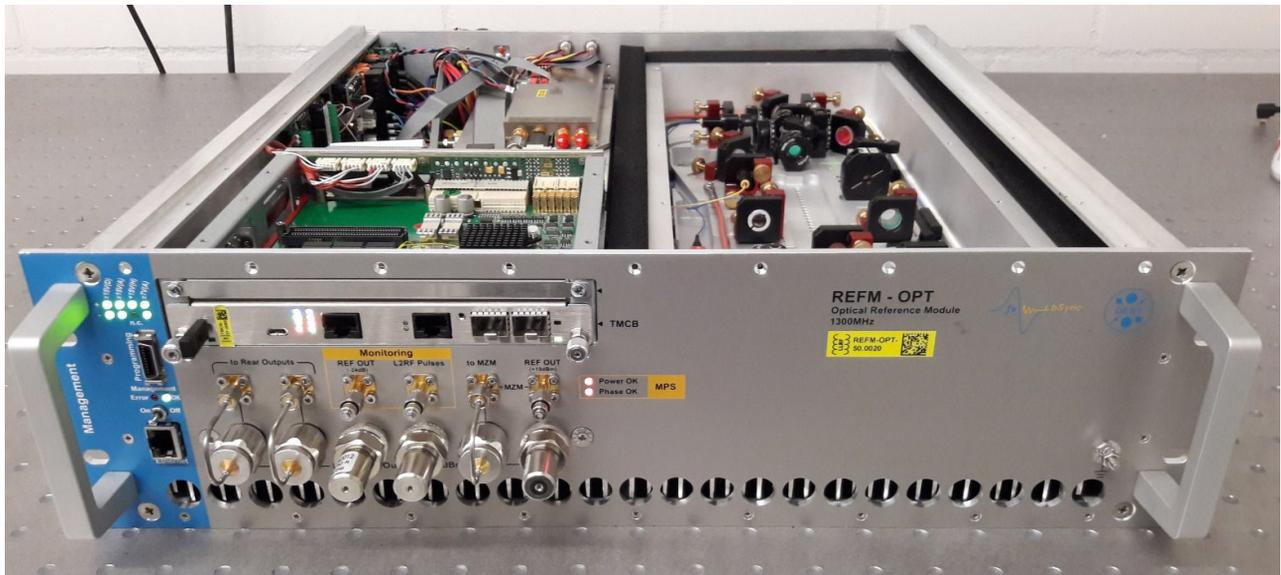
Figure 1: Final REFM-OPT module. On the right hand side the open optical compartment with free-space and fiber optics is visible. On the left hand side the TMCB is mounted on the frontpanel. The outputs from the RF splitter can be found below. The blue part of the front panel features the management and control unit FRED. The L2RF readout electronics, the REACT and the REFMPMS are stacked in the rear.
