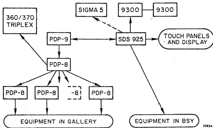
FIG. 2--A map of computer links for increased I/O interface capacity.
