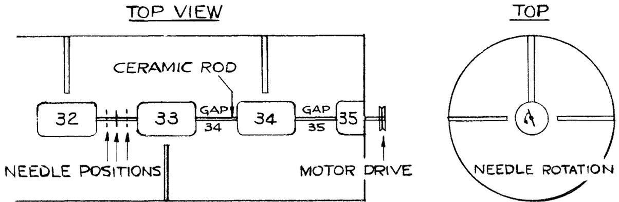
Fig.7. Experimental Setup for Measurement of Transverse Fields
