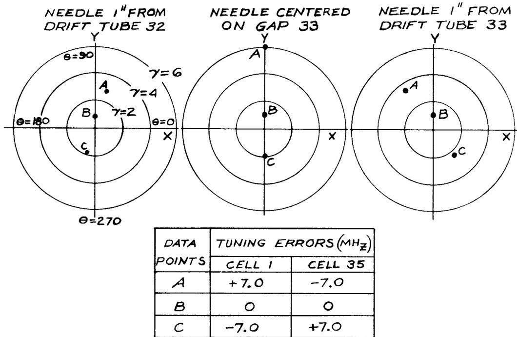
Fig.10. Polar Plot of Transverse Field Data for Structure with Post Couplers
