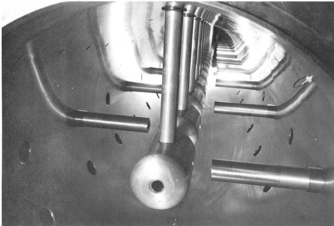
Fig.1. Post Coupled Drift Tube Linac Structure
