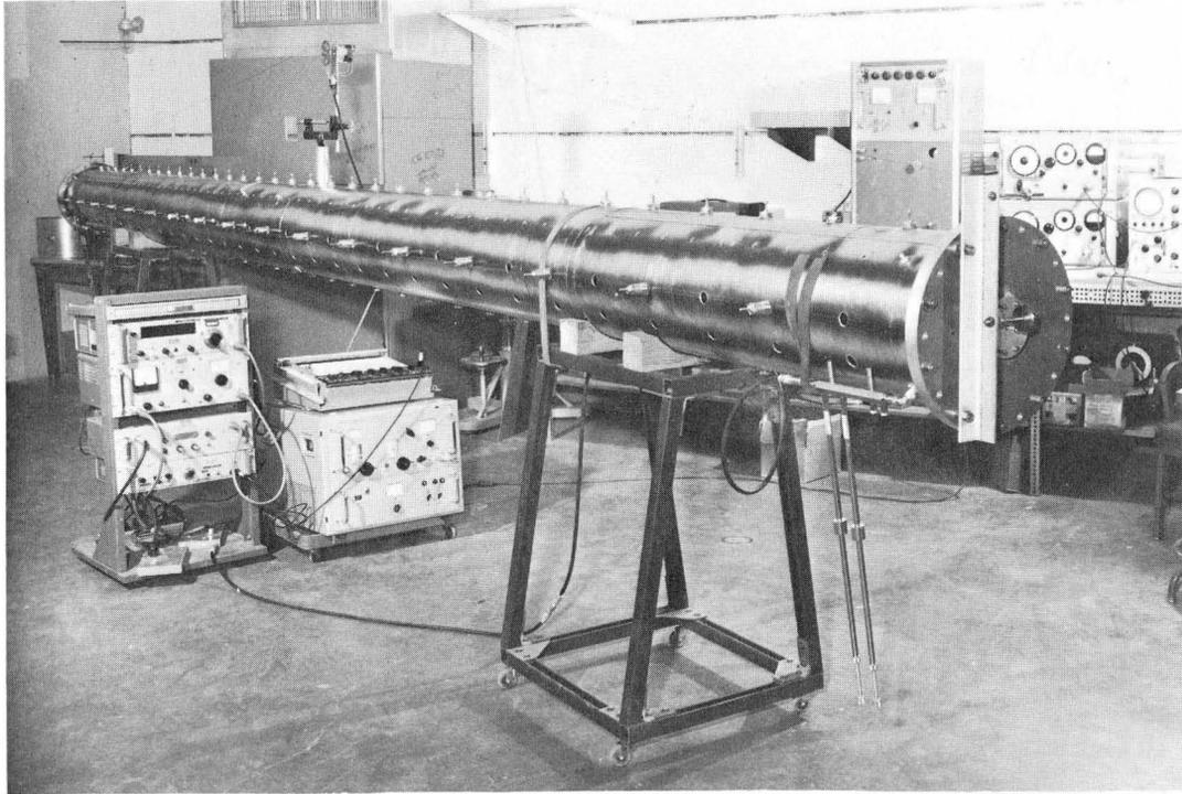
Fig.2. 35-Cell Post Coupled Drift Tube Linac Model
