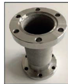
Figure 5: DN40CF tubes in 316L stainless steel by AM.
