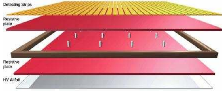
Figure 1.16: Layout of a CMS Resistive Plate Chamber.
