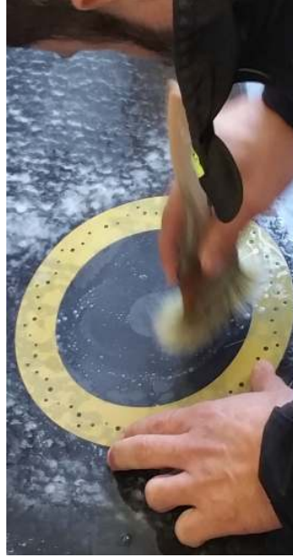
Figure 5.78: Cleaning of the FTM PCB foils: the foil is washed with water and a industrial soap, scrubbed with a brush and then rinsed.
