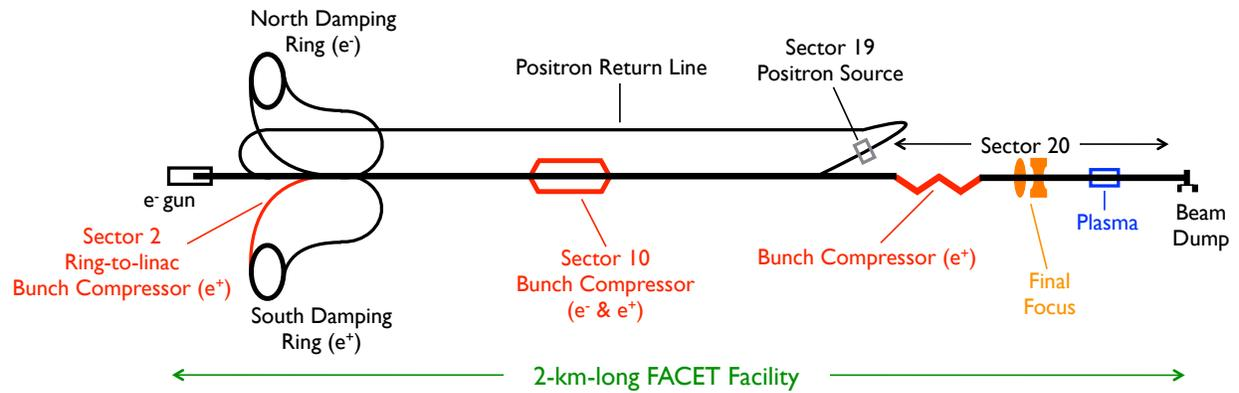
**Extended Data Figure 4 | Schematic of the FACET facility.** Positrons are created in the positron source of Sector 19, transported to the start of the linac by the Positron Return Line, and cooled in the South Damping ring. They are then accelerated in the linac and compressed in the ring-to-linac section, in Sector 10 and in Sector 20, and are focused by the final focus system to the entrance of the plasma in Sector 20.
