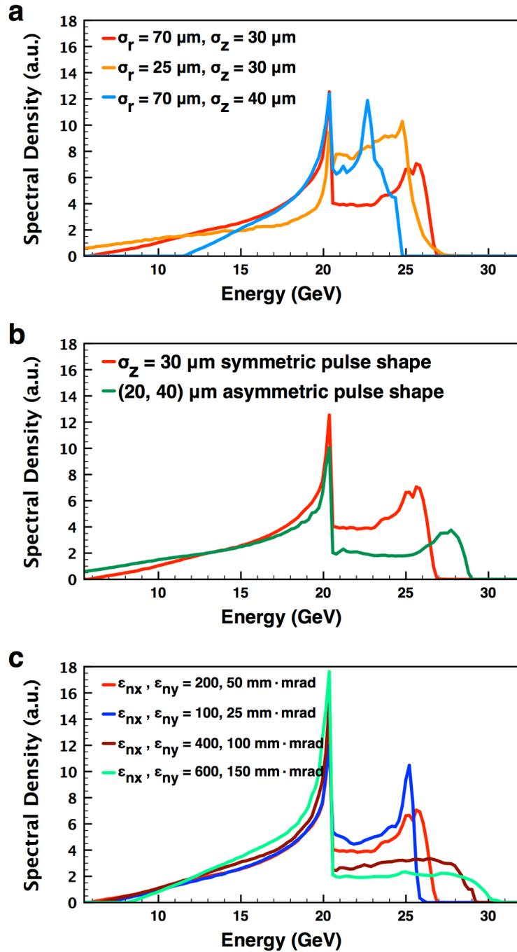
**Extended Data Figure 2 | Sensitivity to bunch parameters in computer simulations.** **a**, Final positron spectrum from QuickPIC simulations as  $\sigma_z$  and  $\sigma_r$  are varied. **b**, Final positron spectrum as the bunch longitudinal asymmetry is varied. The red (green) curve corresponds respectively to a longitudinally symmetric (asymmetric) bunch. **c**, Final positron spectrum as the normalized transverse emittance is varied, holding  $\sigma_r$  constant.
