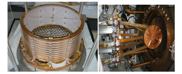
**Figure 1:** Left: One half of the EXO-200 TPC. Right: The fully instrumented liquid xenon vessel being inserted into the cryostat in January 2010.
