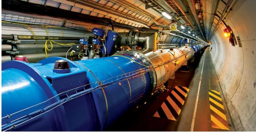
FIGURE 1.1: The Large Hadron Collider (LHC), a 14 TeV center-of-mass energy proton-proton collider in Geneva, Switzerland. Image courtesy of <https://home.cern/topics/large-hadron-collider>.
