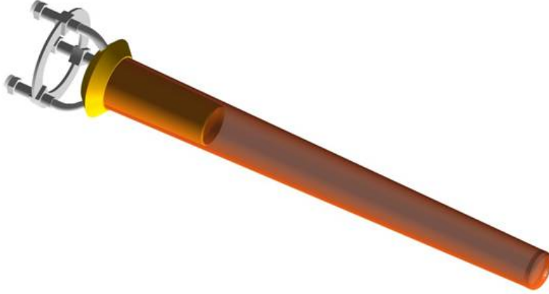
Fig. 3.18. Liquid-deuterium target cell. Picture taken from [34].
