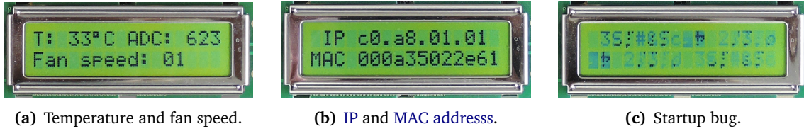
Figure C.1: Two examples of using the LCD which is mounted on the ML605 board. Figure C.1(c) shows the startup bug of improperly addressed cells resulting in character noise.
