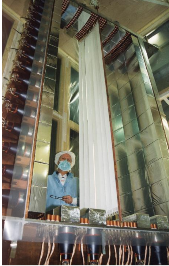
Figure 4.5: A NEMO-3 sector containing a Tellurium source. Optical modules consisting of coupled scintillator blocks and photomultiplier tubes are visible, along with the copper tubes comprising the cathode for the tracking cells [70].
