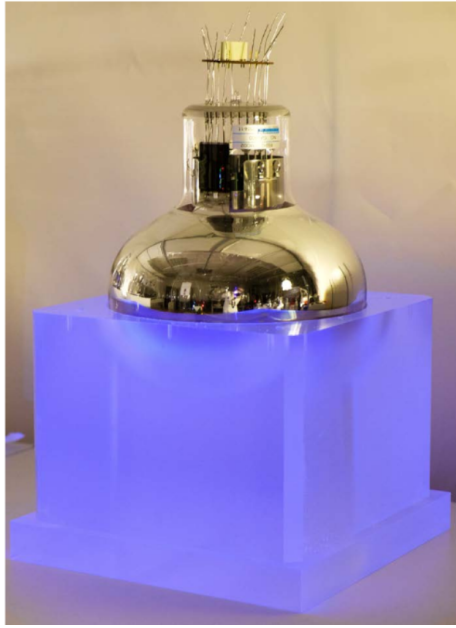
Figure 4.9: Photomultiplier tube directly coupled to a scintillator block.
