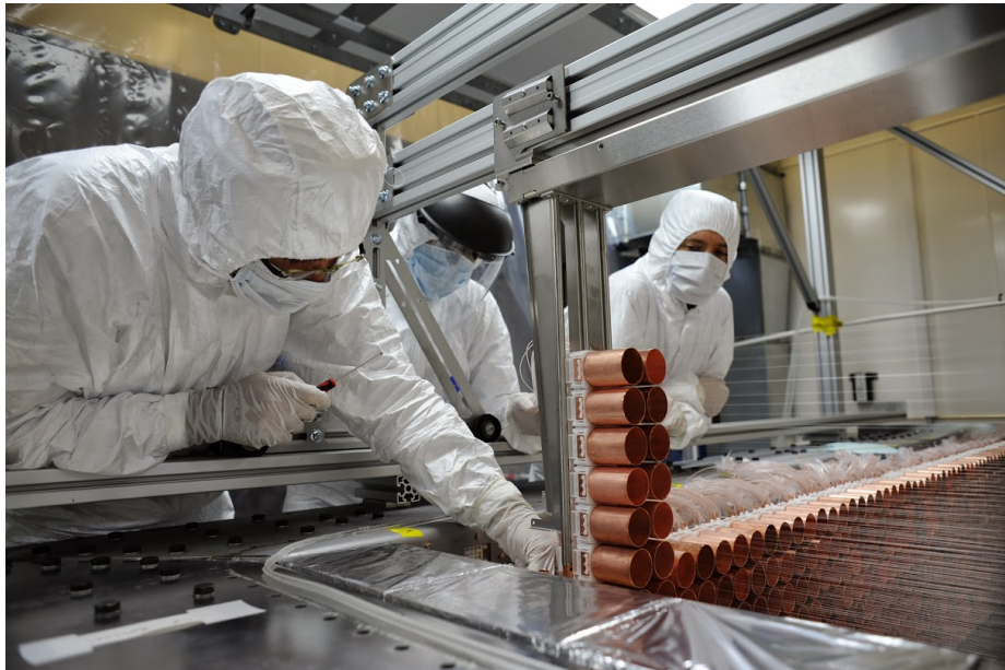
Figure 5.1: A cassette of SuperNEMO Geiger cells being inserted into a tracker section.
