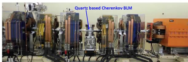
Figure 14: The installation of a quartz based Cherenkov beam loss monitor.
