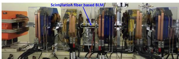
Figure 13: The installation of a scintillation fiber based beam loss monitor.
