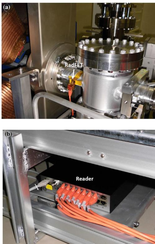
Figure 9: (a) A RadFET and (b) RadFET reader are installed in the inside-wall chamber and cable tray of the storage ring.
