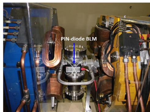
Figure 2: The setup of a PIN-diode BLM.
