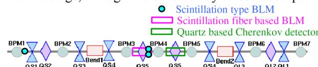
Figure 11: The setup of scintillation and Cherenkov BLMs in the first cell below the injection straight.
