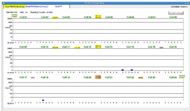
Figure 4: The graphical user interface of PIN-diode BLMs.
