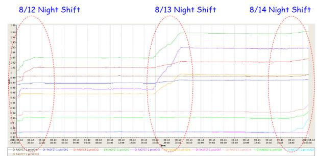
Figure 7: The archived data of the threshold voltages of RadFETs installed in the LTB during the Linac and LTB commissioning from July 12<sup>th</sup> to 14<sup>th</sup>, 2014.
