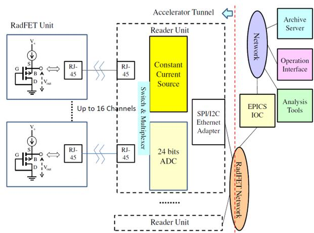
Figure 5: Block diagram of the RadFET setup.
