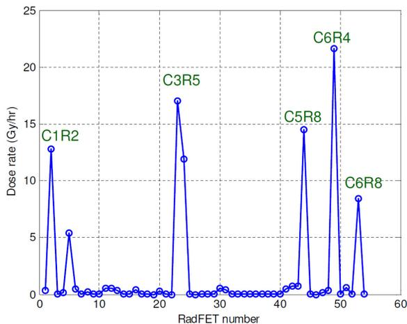
Figure 8: The beam loss pattern as the energy was ramping from 150 MeV to 3 GeV in January 19<sup>th</sup>, 2015.
