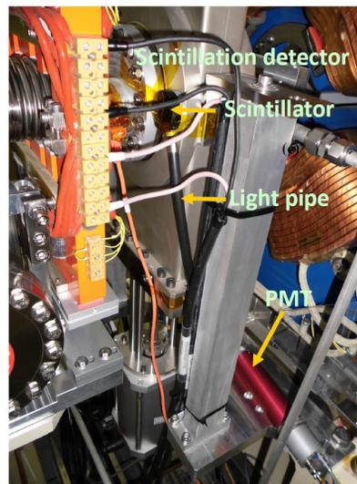
Figure 12: Installation location of a scintillation detector.
