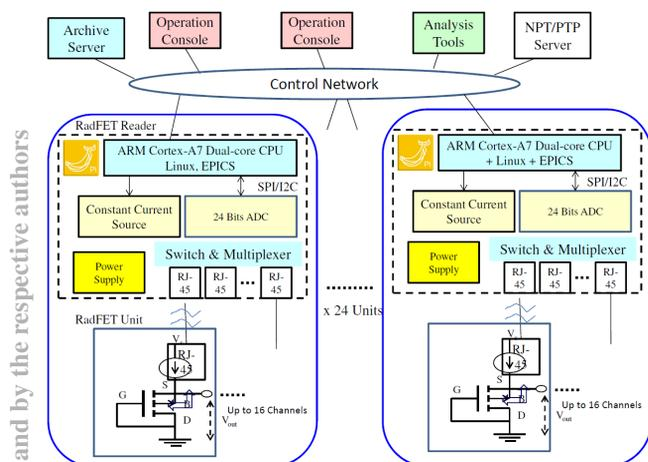
Figure 15: The configuration of the second-generation reader of the RadFET.
