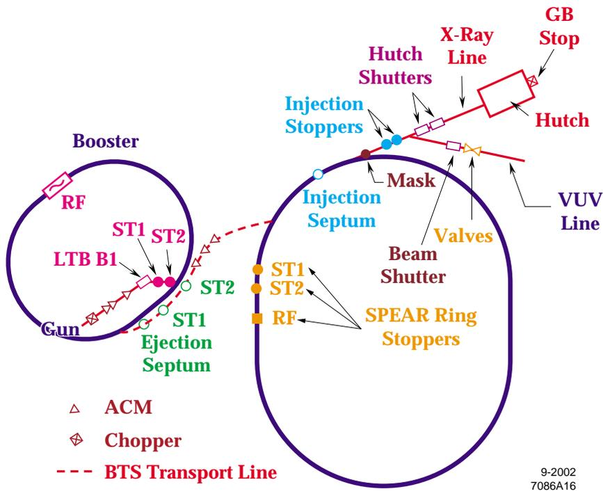
Fig. 3. Main components of the radiation safety system for the SPEAR injector and the ring and a typical synchrotron radiation beam line.
