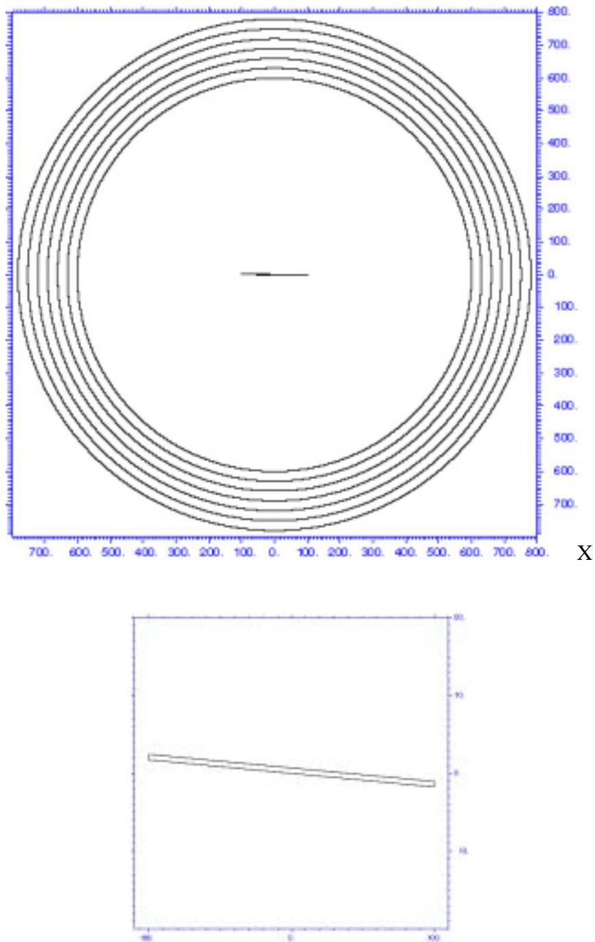
Fig. 4. FLUKA cylindrical shield geometry (top figure) for the generic calculation of SPEAR3 ring shielding design. The 180-cm-thick concrete shield starts at the radius of 600 cm. Electron beam (3 or 5 GeV) direction is +X axis and it hits the target plate at (0,0,0) with the target plate tilted at  $1^\circ$ . The bottom figure shows the 0.7-cm thick copper target plate. The dose is scored as a function of angle and shield depth at the median plane ( $Z = 0$  cm) [10].
