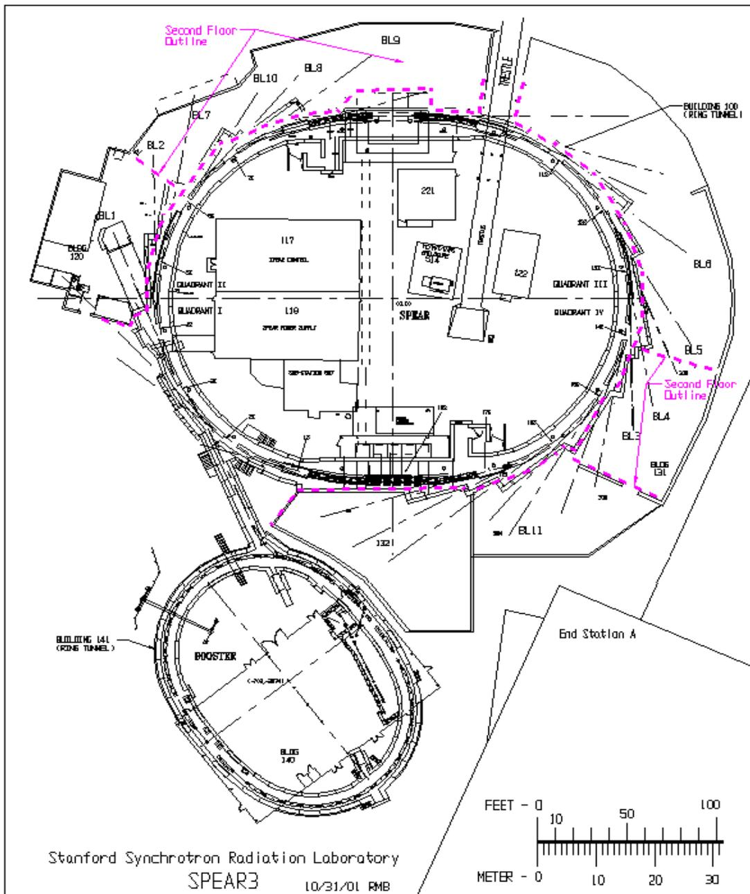
Fig. 1. The SSRL layout, showing the injector (10-Hz, 150-MeV Linac and 3-GeV Booster ring), 234-m-circumference, 3-GeV SPEAR3 ring, and synchrotron radiation beamlines, as well as the building contour around the outer rim of the ring and the 2<sup>nd</sup> floor offices (red dashed line).
