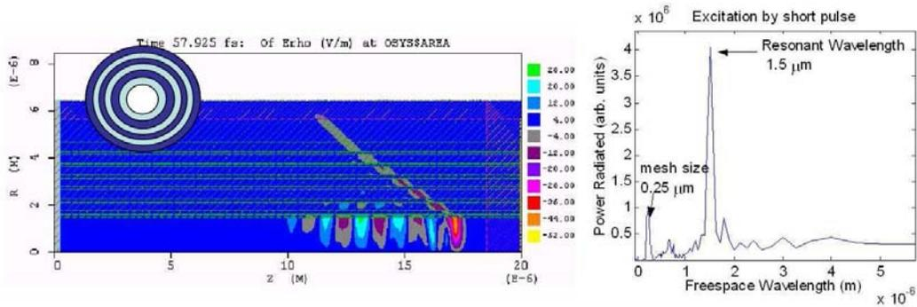
Figure 1: 2D simulation of the wake generated in a Bragg fiber. Left: Snapshot of  $E_r$  in the fiber. Note the Cherenkov angle within the bulk dielectric and the wake generated. The inset shows the cross-section of the fiber. Right: Fourier transform of the on-axis  $E_z$  field showing the resonance at the expected wavelength of  $1.5\mu\text{m}$ .
