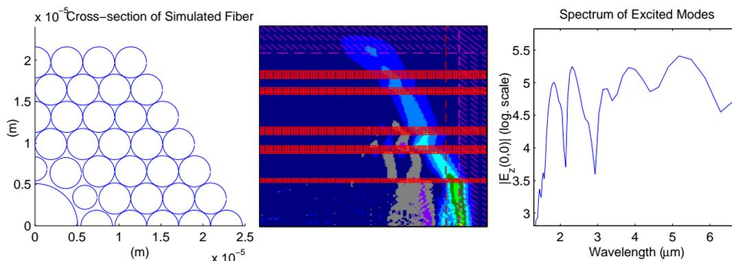
Figure 2: Left: Approximated cross-section of HC-1550 used in simulation. Center: Snap-shot of  $E_z$  field produced by beam traversing fiber. Right: Resulting spectrum excited by the electron beam.
