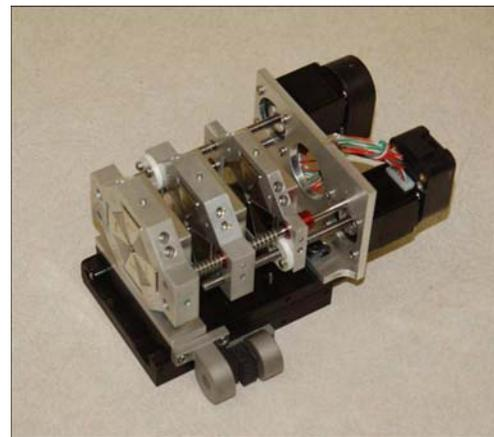
Figure 3: The Permanent Magnet Quadrupole triplet. The first two quads are movable by stepper motor to adjust the final focus, as is the assembly as a whole.
