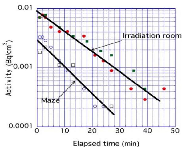
The dose rate of irradiated water, obtained using a NaI (Tl) survey meter, was found to be two times higher than the background level (0.08  $\mu\text{Sv/h}$ ). A very small annihilation peak was observed using a LaBr<sub>3</sub>(Ce) spectrometer. It was concluded that the structure material of water phantom was slightly activated.
