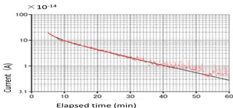
Activities of the filters collected from the irradiation room and the maze to the irradiation room were also measured, and the half-life of the radioactive substance detected was about 10 min in the irradiation room, as shown in Figure 3. Activity concentration was  $0.009$  and  $0.003 \text{ Bq}\cdot\text{cm}^{-3}$  at the end of irradiation in the irradiation room and the maze. An aerosol of radioactive nitrogen oxide ( $\text{NO}_x$ ) may have been produced by the radiation effect.
