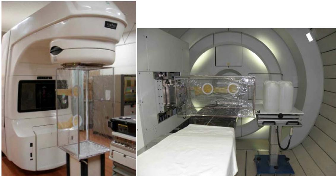
A portable air sampler with a set of HEPA filter (HE-40T) (collection efficiency: 99.6%, particle size 0.09 to 0.8  $\mu\text{m}$ ) and charcoal filter (CP-20) was used for aerosol sampling in the irradiation room and the maze to the irradiation room during irradiation. Radioactivity collected on the filter was measured using a GM survey meter (window size: 50 mm $\phi$ , TGS-146, Aloka Co.).
