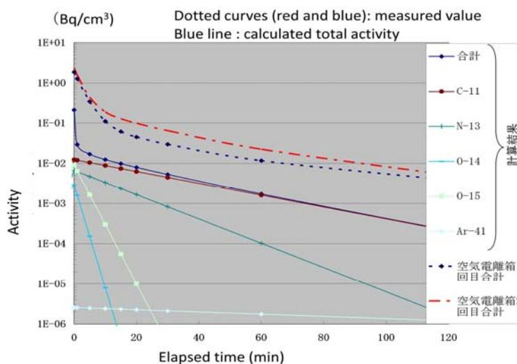
The activities of the filters collected from the irradiation room and the maze to the irradiation room were also detected and the half-life of these activities was 10 min. The activity concentration was lower than that of proton irradiation. At the end of irradiation, the activity concentration was about  $0.02 \text{ Bq}\cdot\text{cm}^{-3}$  in the irradiation room.
