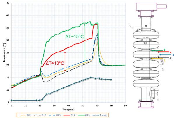
Figure 3: Temperature measurements on cavity central cell surface during BCP, different colours correspond to different location as depicted in the sketch on the right.
