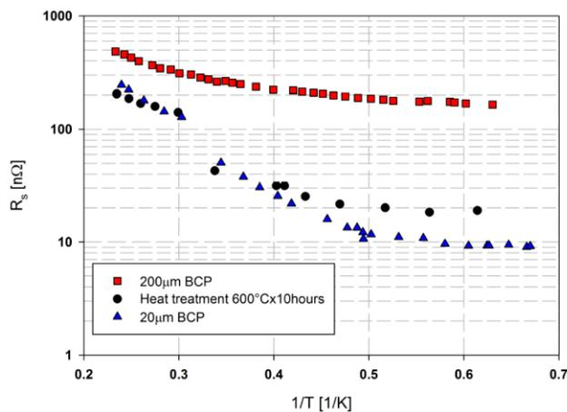
Figure 6: P01 surface resistance with respect to temperature at different preparation phases.
