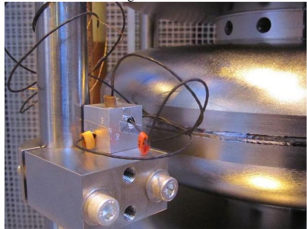
Figure 7: Fluxgate probes installed near the cavity surface in the equator region.
