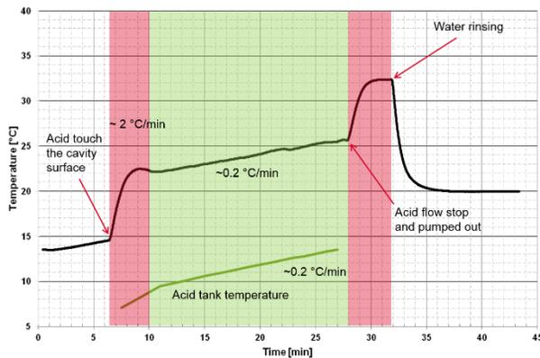
Figure 2: Temperature measure on cavity surface during BCP.
