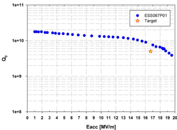
Figure 5: Vertical test #4 cavity P01 performance exceed requirements.
