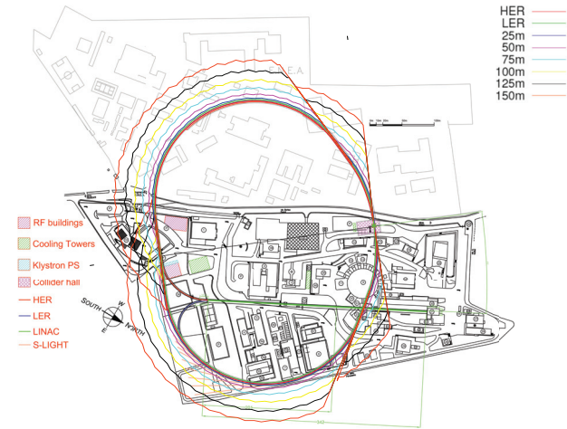
Figure 4: All possible bend magnet photon beam line location with different contour lines showing the distance to the source point.
