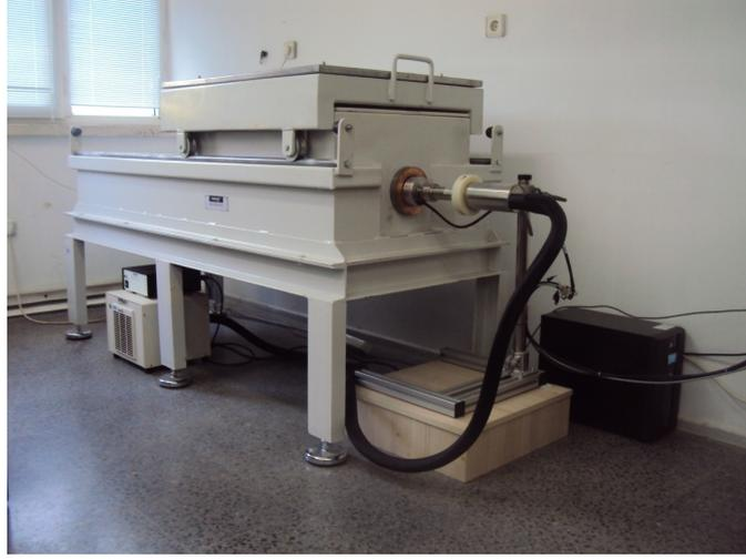
Figure 4.3: HPGe detector setup used in this work.
