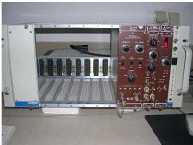
Figure 2.2: Typical NIM-based electronic setup
