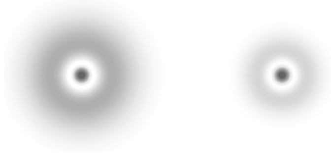
Fig. 7. The planar magnetic field, displayed in terms of r/r_0 for r_0 = 0.5 (left) and 1 (right).
